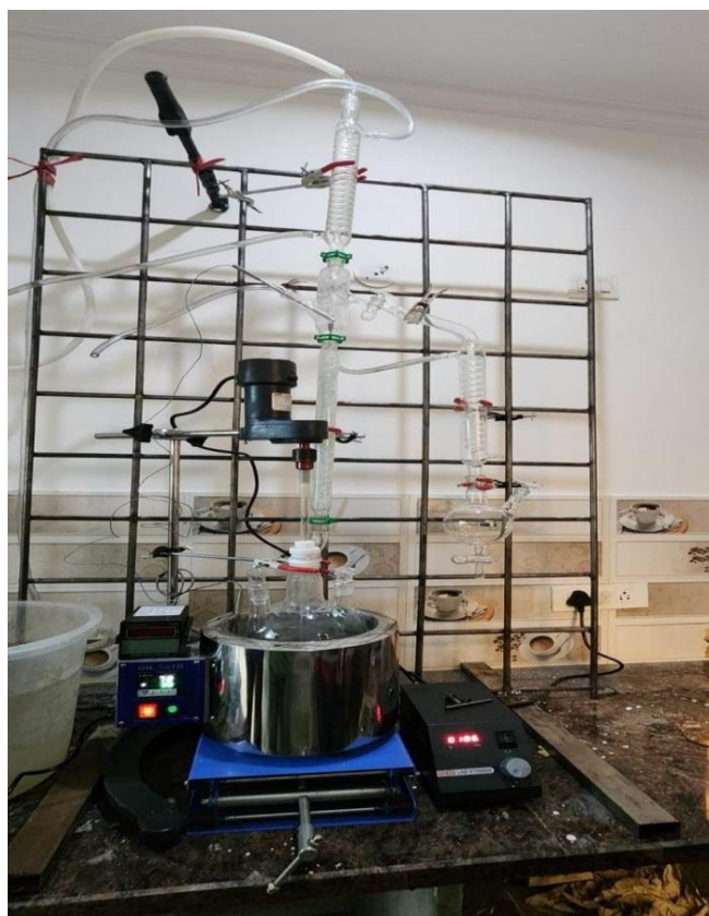
Fig 4 Experimental setup for catalytic conversion of waste plastic into diesel-range fuel,
