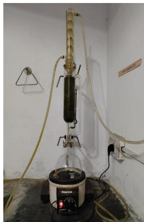
Figure 3: Continuous Hot Extraction Process
